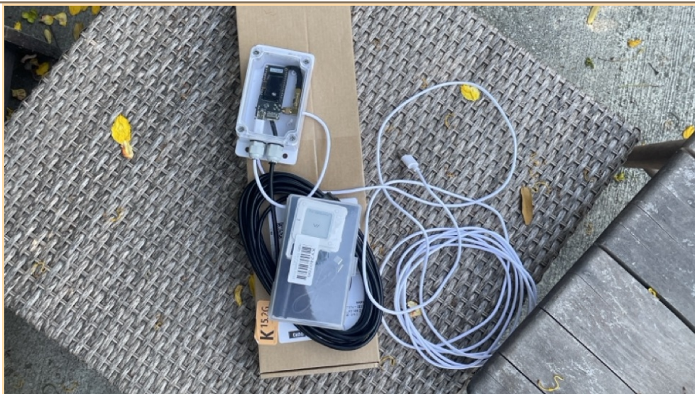
Top: LILYGO T3-S3 in enclosure. Bottom: LILYGO T-Echo. Underneath, inside the cardboard box: Fiberglass antenna. – Photo by KK6JBU
